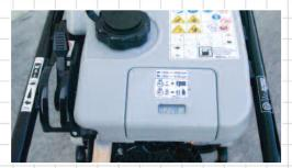
New on-board hourmeter/tachometer. allows accurate tracking of usage and maintenance intervals. With its new recoil guard the MTX range are also protected from impact damage eliminating costly repairs and downtime.
